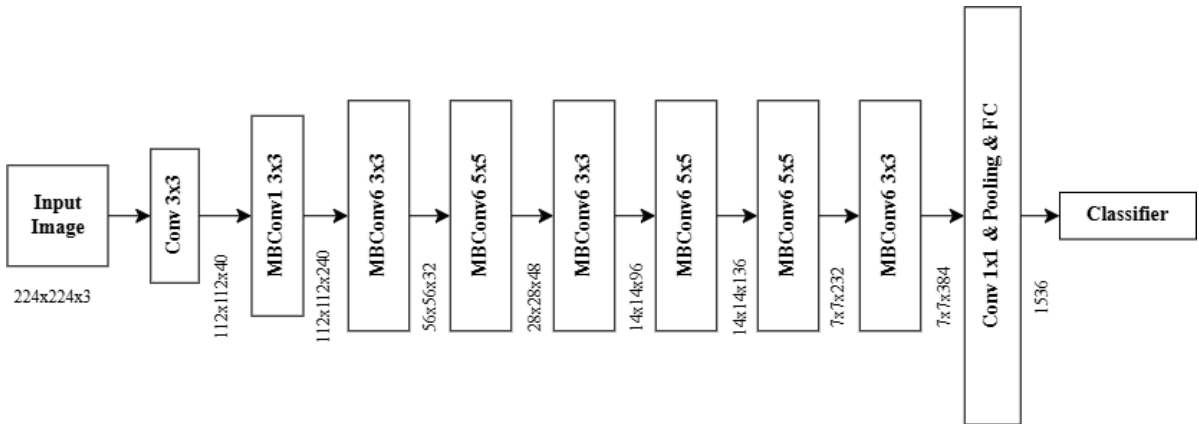
Fig 17. Efficient Net-B3 architecture
